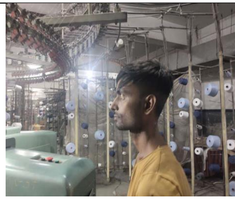
NC Photo-3- Workers not wearing ear plug in Knitting section.
