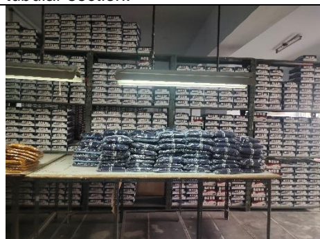
NC Photo-4- Packed cartons stacked at unsafe height in warehouse section on ground floor.
